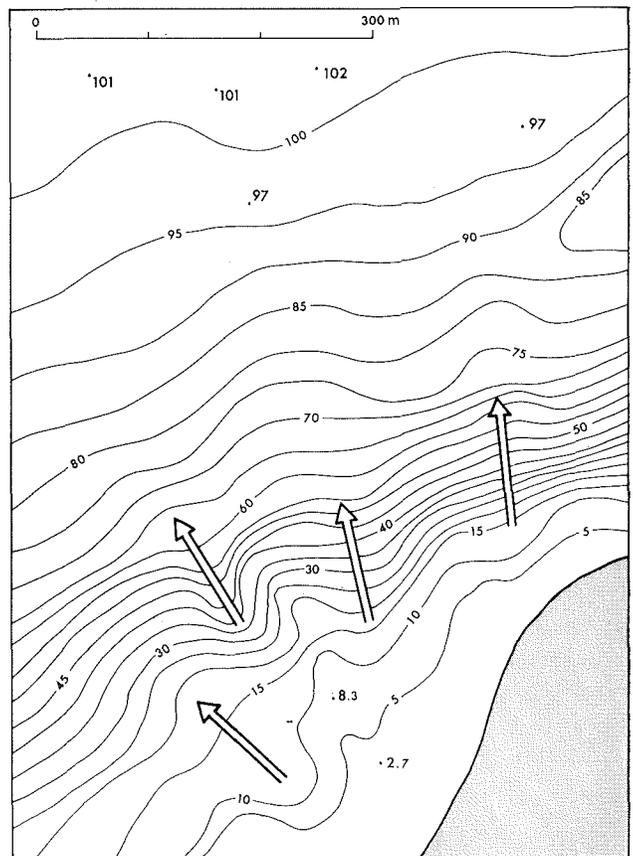
Fig. 12. Map of the submarine slope off the western shore of the northern ness based on 1967 soundings. Avalanche scars (arrows) in the upper part of the slope and debris tongues at its base.
