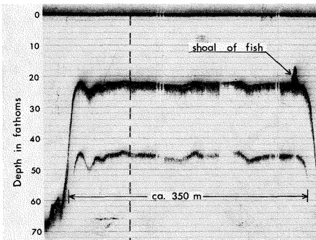
Fig. 11. Echogram of the Surtla shoal from WSW-ENE recorded on June 28, 1968. According to soundings of July 1967 (cf. Fig. 1) waves and currents have lowered the plateau from 18 to 22 fathoms in one year.
